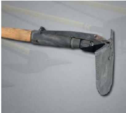
Caption: A typical combi tool configured in this example as a hoe.
