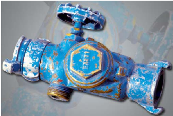
Caption: A typical check and bleeder valve.
