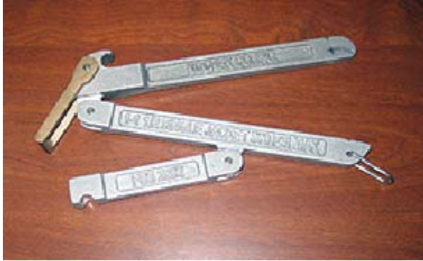
Caption: An example of a typical forestry hose clamp.
