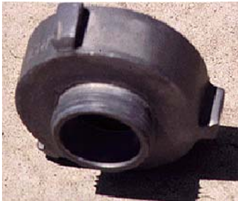
Caption: An example of a reducer/increaser.
