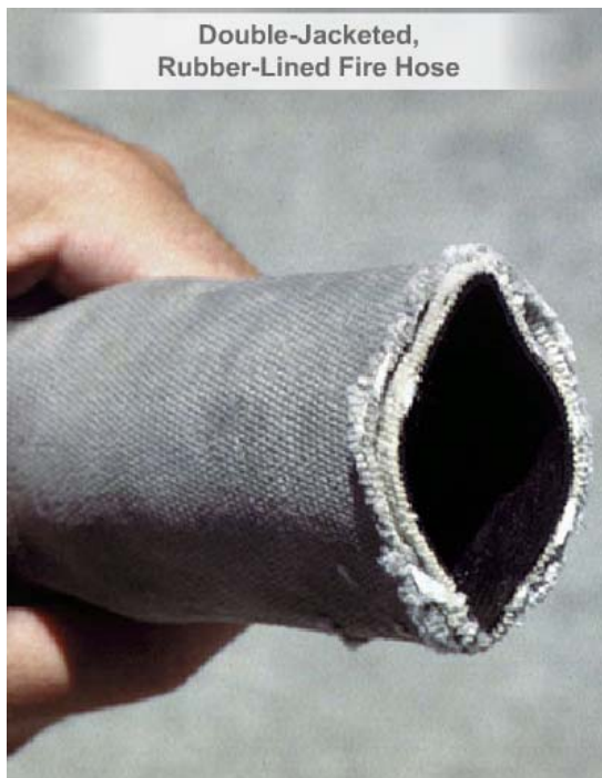
Caption: A cross section of a jacketed, lined rubber hose.
