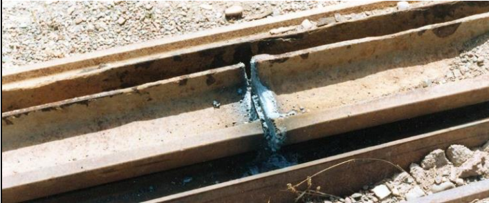
Evidence of oxyacetylene cutting
