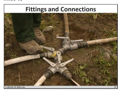
• Deploying hose further than 50 to 100 feet requires fittings and connections.
